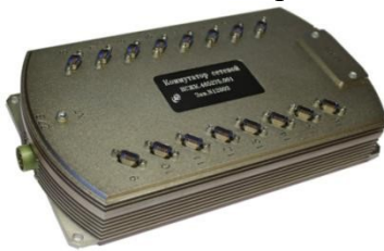
Fig. 6. 16-port SpaceWire routing switch for airborne networks
